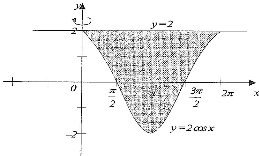
A mathematically inclined microwave cooking enthusiast decided to design his own cake pan. The shape of the interior of the cake pan is obtained by rotating the region bounded by the curve  $y = 2 \cos x$ ,  $0 \leq x \leq 2\pi$  and the line  $y = 2$  through  $360^\circ$  about the  $y$ -axis. Use the method of cylindrical shells to show that the volume of the
